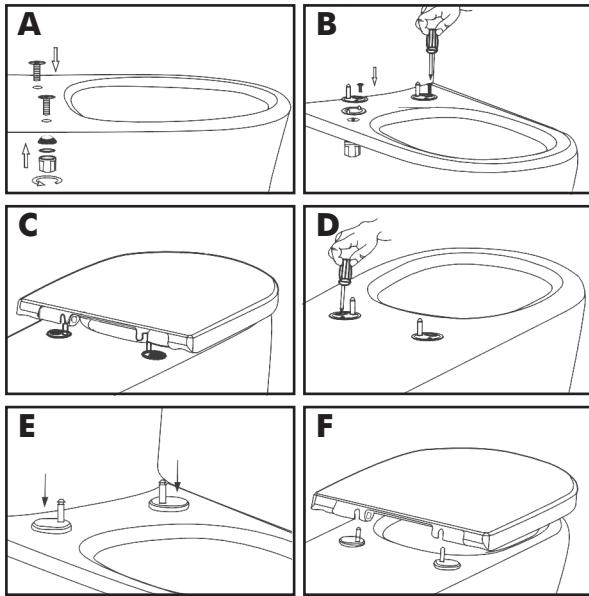
A) First, put the nylon screws (5) into the holes, as illustrated. Then place the rubber ring (6), add the nylon washer (7) and tighten the nylon nut (8) in place.
