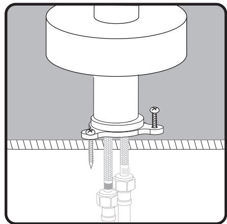
As illustrated, screw or firmly anchoring the base flange (14) firmly on the floor put in place the base flange cover (12)
