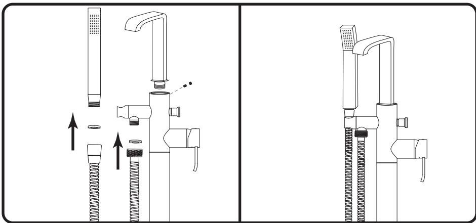
Place the spout (1) in position and secure it with the Allen screw (9), add the finishing cap (10). Connect flexible hoses (17) to the hand shower (13) and the faucet (1), make sure the rubber washers (14) are in place. Carefully align the threads, hand tighten firmly. **Do not use a wrench or pliers.**
